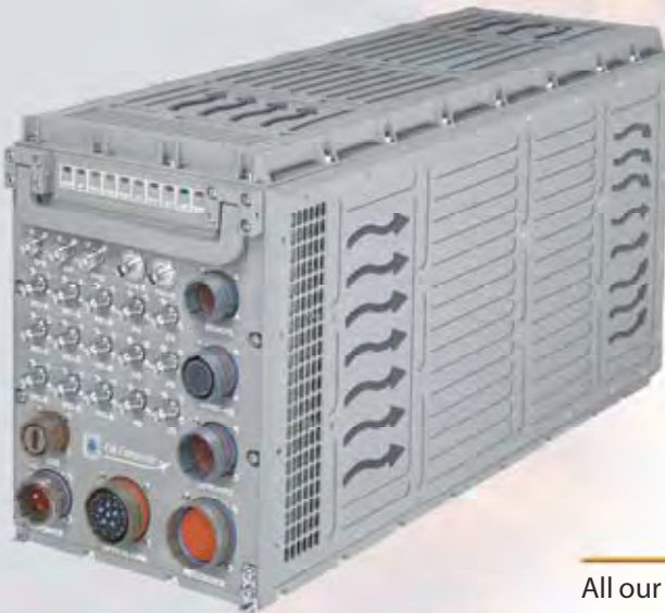
Sealed 3/4 ATR, 7 slot, 800 W PSU, +5V (+3.3V) 80 A, 14 Kg
