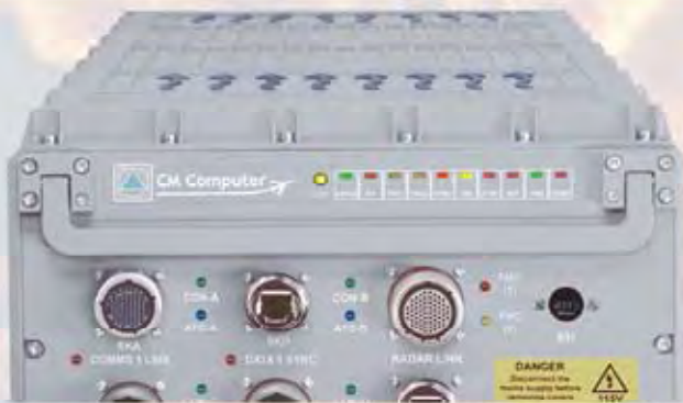
Sealed 1 ATR, 12 slot, 1500 Watts PSU, +5V (+3.3V) 160 Amps, 17 Kg
